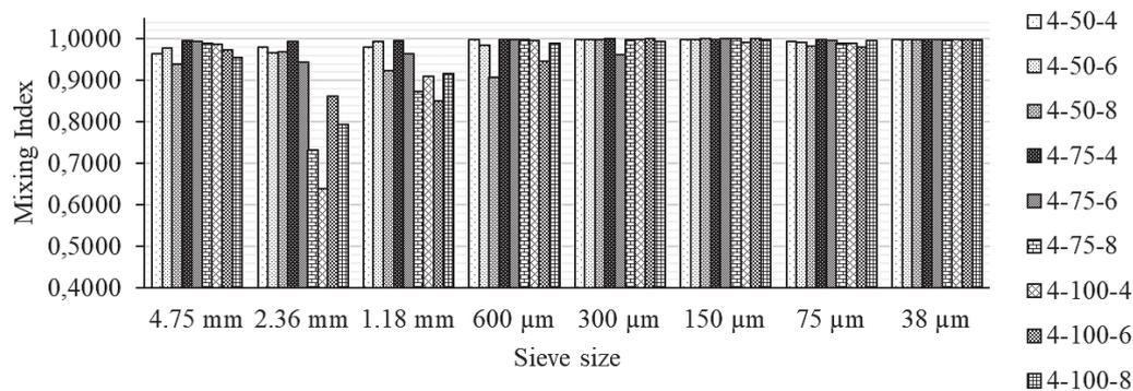
Fig. 6. The relationship between particles at mesh size 4 mm and mixing index at different mixing speed and times
