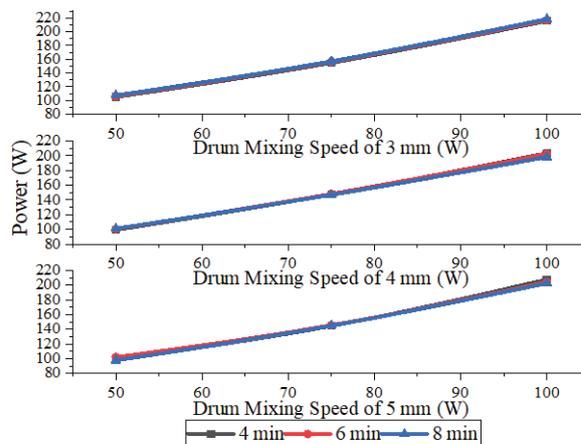
Fig. 8. The power of mixing shaft in mixing the particles passed through mesh sizes 3 mm, 4 mm and 5 mm
