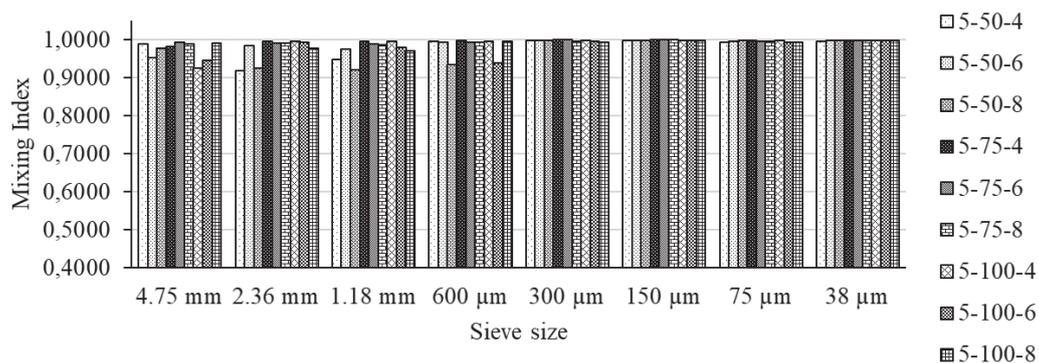
Fig. 7. The relationship between particles at mesh size 5 mm and mixing index at different mixing speeds and times
