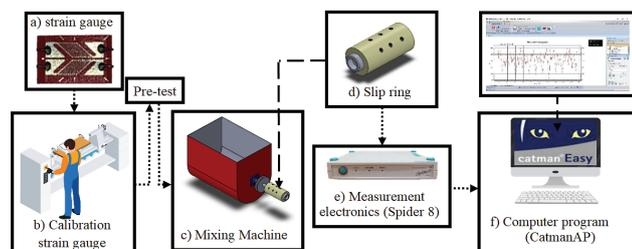
**Fig. 4. Power consumption in mixing**
