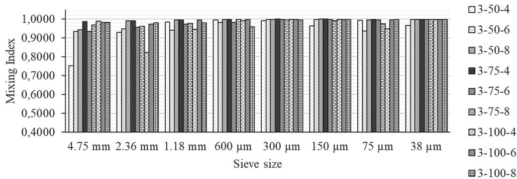
Fig. 5. The relationship between particles at mesh size 3 mm and mixing index at different mixing speed and times
