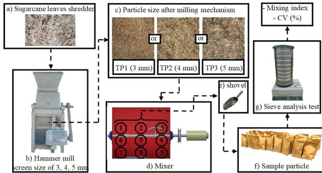
Fig. 2. Particles mixing testing method
