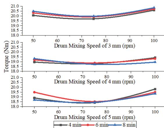
Fig. 9. Torque of mixing shaft in mixing the particles passed through mesh sizes 3 mm, 4 mm and 5 mm
