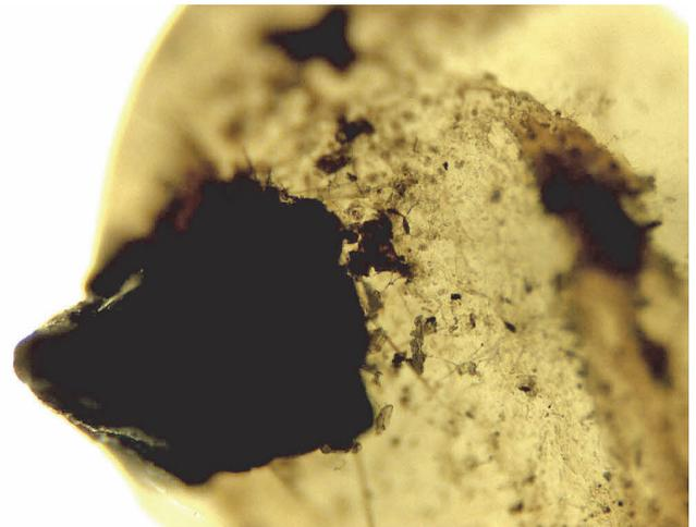
**Fig. 4. Sesame seed threshed by threshing apparatus of grain harvester**
