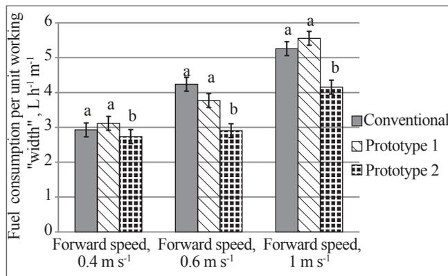
**Fig. 2. Fuel consumption of machines**
