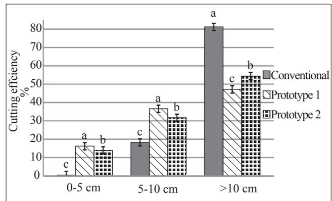
**Fig. 5. Cutting efficiency of machines at a forward speed of 1 m s<sup>-1</sup>**
