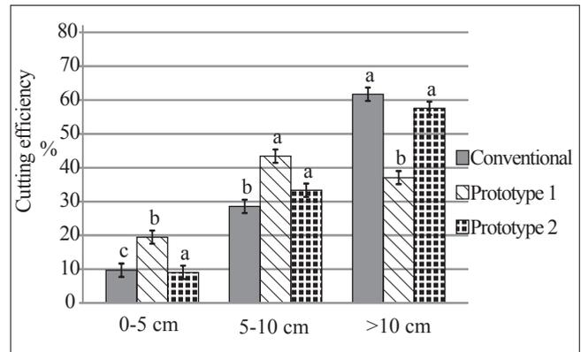
**Fig. 3. Cutting efficiency of machines at a forward speed of 0.4 m s<sup>-1</sup>**
