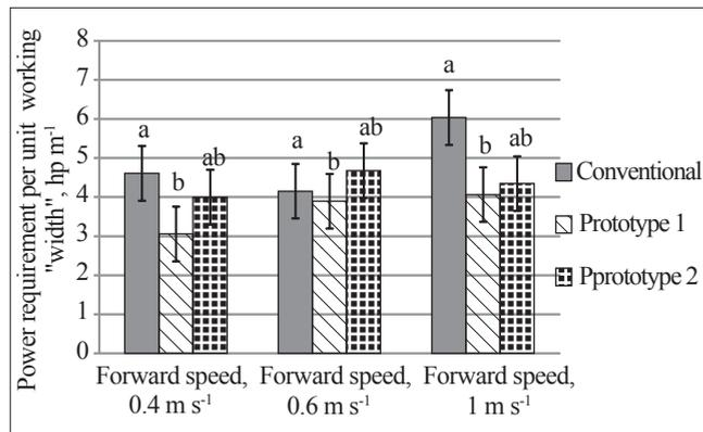
**Fig. 1. Power requirement of machines**
