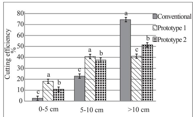
**Fig. 4. Cutting efficiency of machines at a forward speed of 0.6 m s<sup>-1</sup>**
