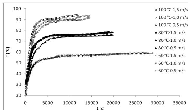
Fig. 3. Experimental temperature values for mixture 2
