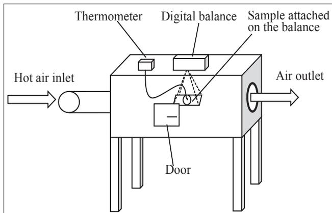
Fig. 1. Schematic sketch of tunnel dryer
