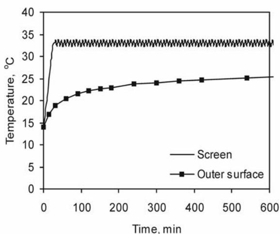
**Fig. 3. Temperature variation of the screen and surface of the heated trap at 14.5 °C temperature of grain**
