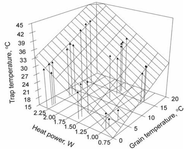
Fig. 2. Temperature of the trap screen at different heater power and grain temperatures
