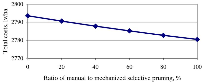
**Fig. 9. Variation of total costs depending on the ratio of manual to mechanized selective pruning**
