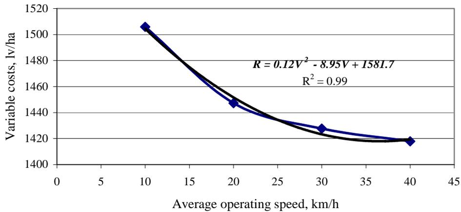
**Fig. 8. Effect of average operating speed on the variable costs during transport operations in grape cultivation and harvesting**
