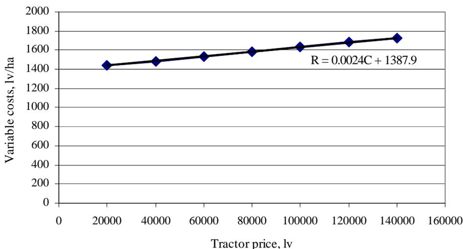
**Fig. 7. Effect of price of the basic power means on the variable costs**
