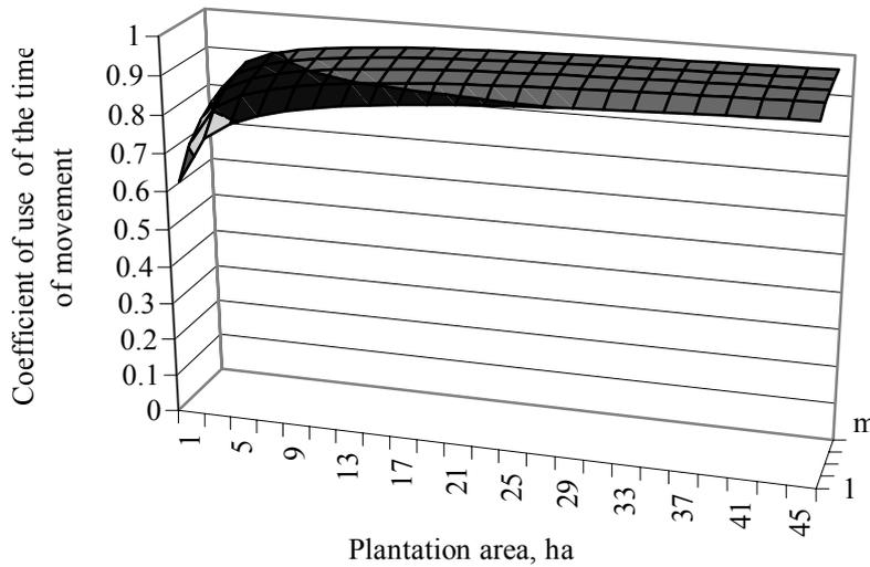
**Fig. 2. Effect of ratio of plantation length to width and plantation area on the coefficient of use of the time of movement**
