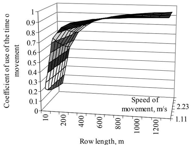
**Fig. 1. Effect of movement speed of the aggregate and row length on the coefficient of use of the time of movement**
