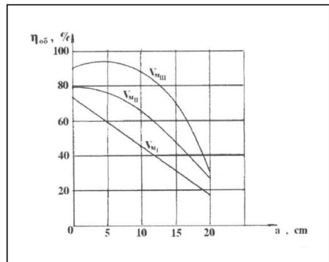
**Fig. 4.** Degree of turning over the soil layer, depending on the working depth
