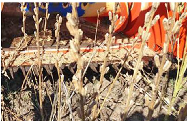
**Fig. 1. Sesame seeds on the cutting apparatus at harvesting with grain harvester**
