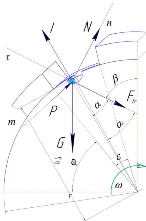
**Fig. 3. Forces affecting a seed when it is transported to the dropping zone**
