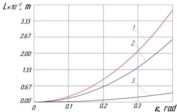
**Fig. 4. Dependences of the movement of the particle along the blade on the rotation angle of the disk under the condition that vacuum is produced at angular velocities: 1 – 30 rad/s, 2 – 25 rad/s, 3 – 20 rad/s**
