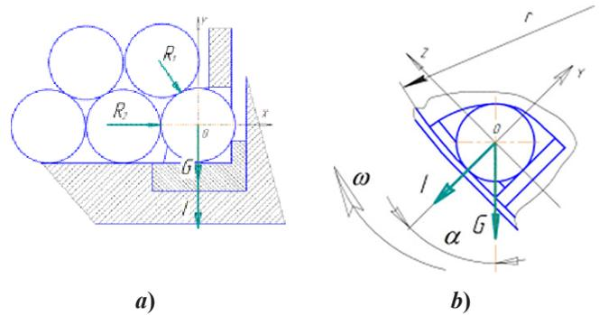
**Fig. 2. Forces affecting a seed in the process of catching: a – layout of forces in projection XOY; b – layout of forces in projection XOZ**
