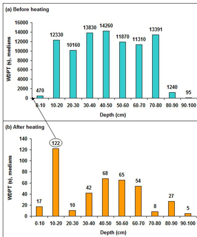
Fig. 1. Water drop penetration time in the soil profile layers (medians)
