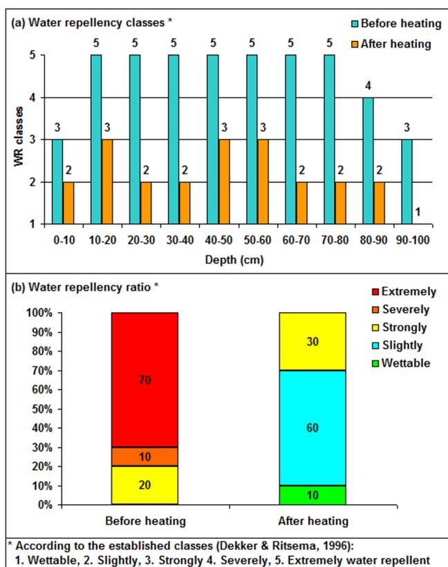
**Fig. 2. Classes and ratio distribution of water repellency in the soil profile**
