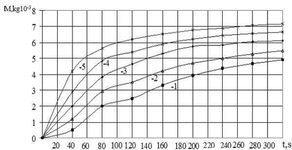
**Fig. 3. Determination of the amount of precipitate in the exciter 1.3 kW and different temperature oil: 1 – 20 °C; 2 – 30 °C; 3 – 40 °C; 4 – 50 °C; 5 – 6 °C, jitter frequency of the ultrasonic irradiator 120 kHz**
