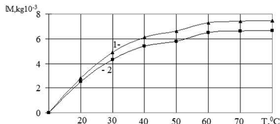
**Fig. 6. Determination of sediment for 200 seconds filtration and change of oil temperature: 1 – the power of ultrasonic vibrations is 1.3 kW; 2 – without using ultrasonic vibrations**
