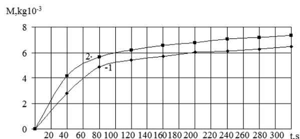
**Fig. 4. Comparative analysis of the precipitate obtained: 1 – without using ultrasonic vibrations, the oil filtration temperature is 55 °C; 2 – use of ultrasonic vibrations. Sonication mode: oil temperature 55 °C with 1.3 kW ultrasonic vibration, ultrasonic wave frequency 120 kHz**
