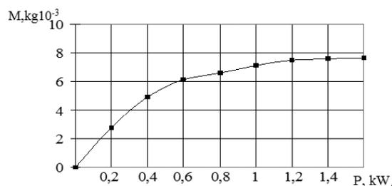
**Fig. 5. Determine the filter cake for 200 seconds at an oil temperature of 55 °C and change the force of ultrasonic vibrations**
