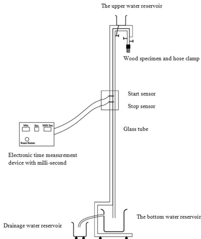
**Fig. 1. The overview of the gas permeability apparatus equipped with milli-second precision electronic time measurement device (USPTO No. 8,079,249 B2; Pub No. 2010/0281951) (Approved by The Iranian Research Organization for Scientific and Technology under certificate No. 47022)**
