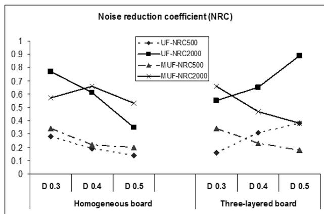
**Fig. 6. Noise reduction coefficients for the 12 treatments in the present study at 500 and 2000 Hz frequencies (UF = Urea Formaldehyde resin; MUF = Melamine Urea Formaldehyde resin; D = Density)**
