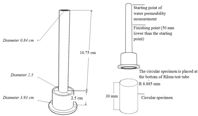
**Fig. 2. Liquid permeability measurement apparatus (Rilem test tube)**
