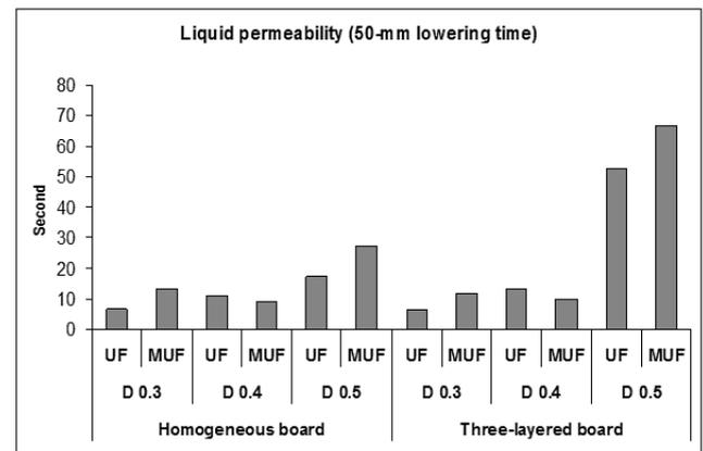
**Fig. 5. Liquid permeability of 50-mm lowering time (second) for the 12 treatments in the present study (UF = Urea Formaldehyde resin; MUF = Melamine Urea Formaldehyde resin; D = Density)**
