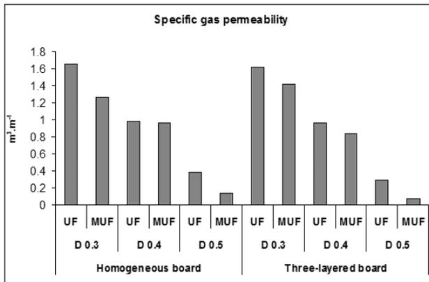
**Fig. 3. Specific gas permeability for the 12 treatments in the present study (UF = Urea Formaldehyde resin; MUF = Melamine Urea Formaldehyde resin; D = Density) ( $\times 10^{-11} \text{ m}^3 \cdot \text{m}^{-1}$ )**
