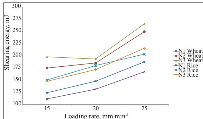
**Fig. 4.** Shearing energy of wheat and rice straw at different internode's positions under 15, 20 and 25 mm min<sup>-1</sup>
