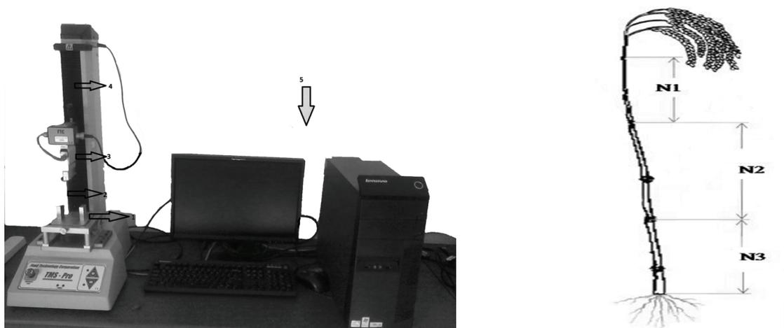
**Fig. 1. a - Configuration of analyzer machine used to measure the mechanical characteristics of wheat and rice straw: 1. Metallic supports; 2. Loading plate; 3. S- type force sensor; 4. Compression mode; 5. Data acquisition system (Computer system attached with machine).
