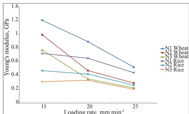
**Fig. 5. Young's modulus of wheat and rice straw at different internode's positions under 15, 20 and 25 mm min<sup>-1</sup>**
