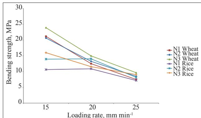
**Fig. 3.** Bending strength of wheat and rice straw at different internode's positions under 15, 20 and 25 mm min<sup>-1</sup>
