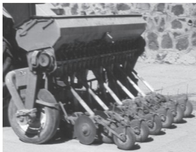
Fig. 1. Seed drill used in the experiment with rubber press wheels
