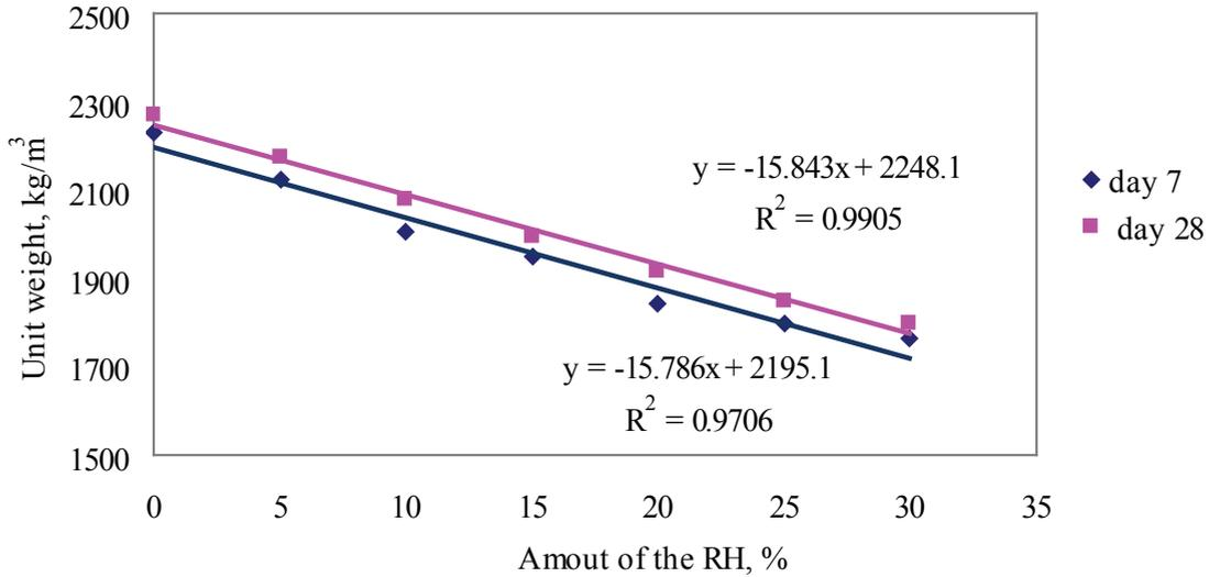
Fig. 2. The unit weight versus the amount of RH
