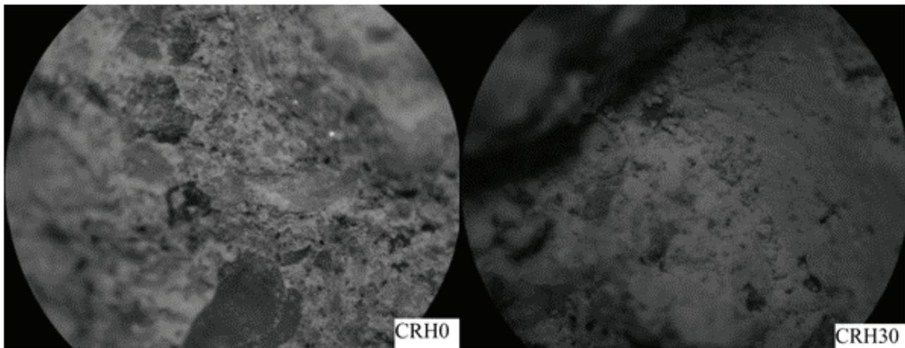
**Fig. 1. The microscopic image of the hardened concretes**
