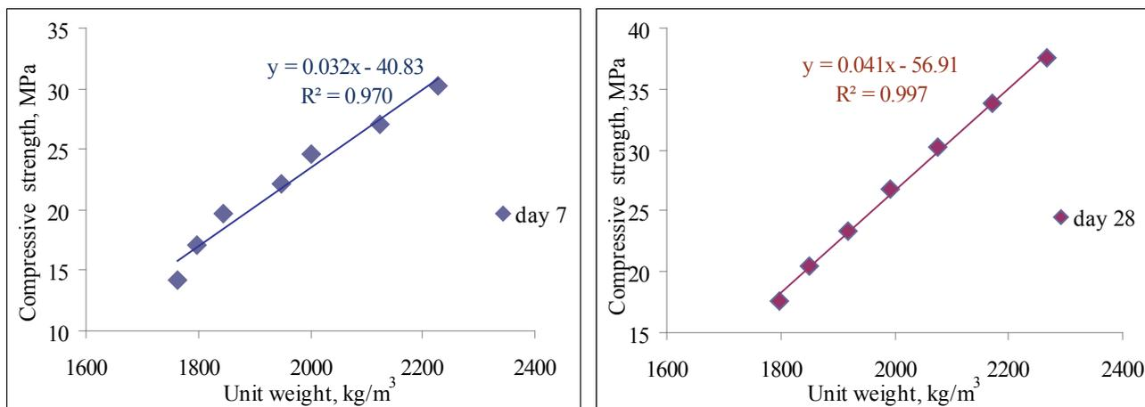
Fig. 4. The compressive strength versus unit weight
