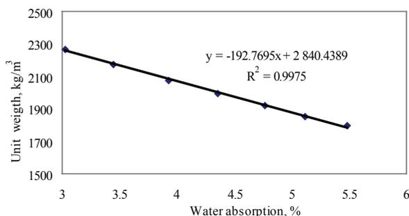
Fig. 5. The relationship between water absorption and unit weight
