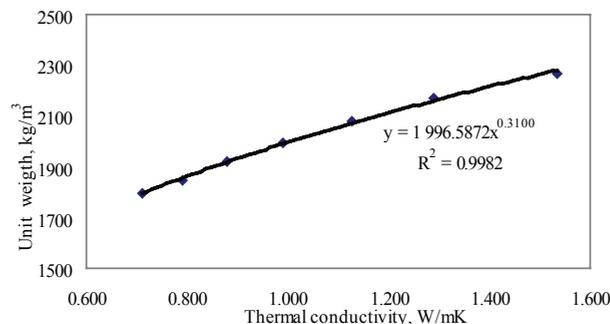
Fig. 6. The relationship between thermal conductivity and unit weight
