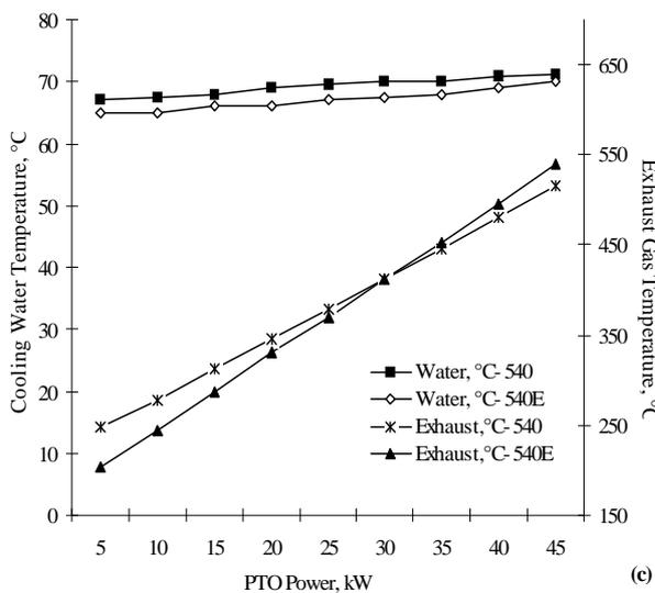
**Fig. 3. Exhaust gas and cooling water temperatures depending on the loads applied to the tractor PTO at 540 and 540E operations (a) JD 5625, (b) MF 3085, (c) NH TD85**
