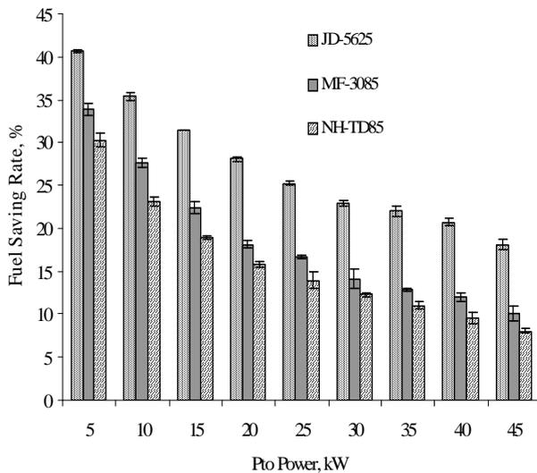
**Fig.2. Fuel saving rates resulting from 540E operation in comparison to 540 operation**
