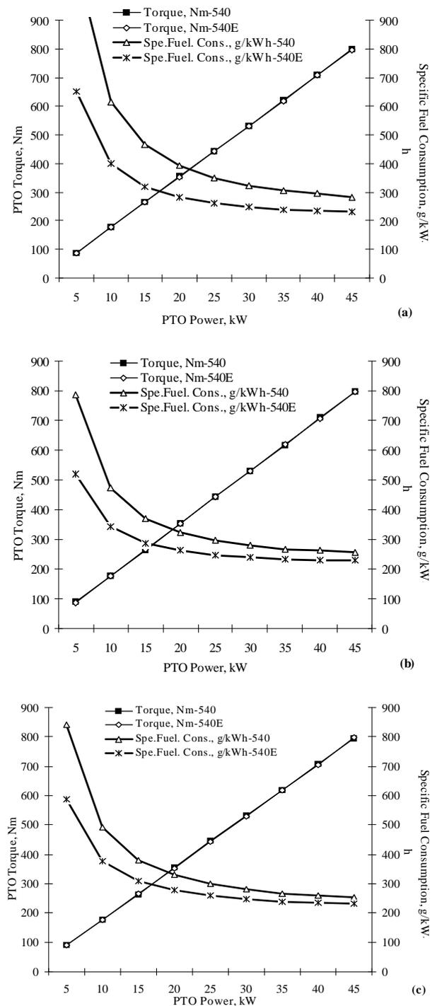
**Fig. 1. PTO torque and engine’s specific fuel consumption depending on the loads applied to the tractor PTO at 540 and 540E operations (a) JD 5625, (b) MF 3085, (c) NH TD85**
